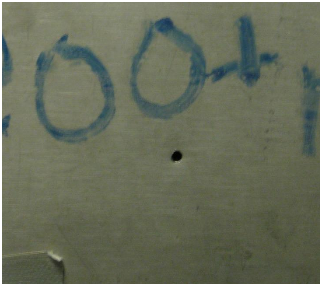
The bullet hole in the CRISAT-panel.
