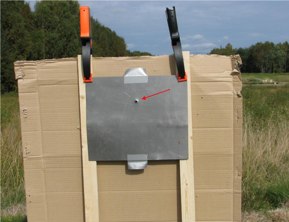
The rear of the test pack, showing the witness plate. The exit hole is indicated by the arrow.
