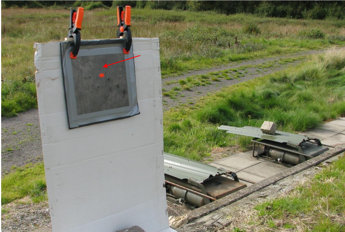
The CRISAT-panel when shot from a distance of 300m. The point of impact is indicated by the arrow.
