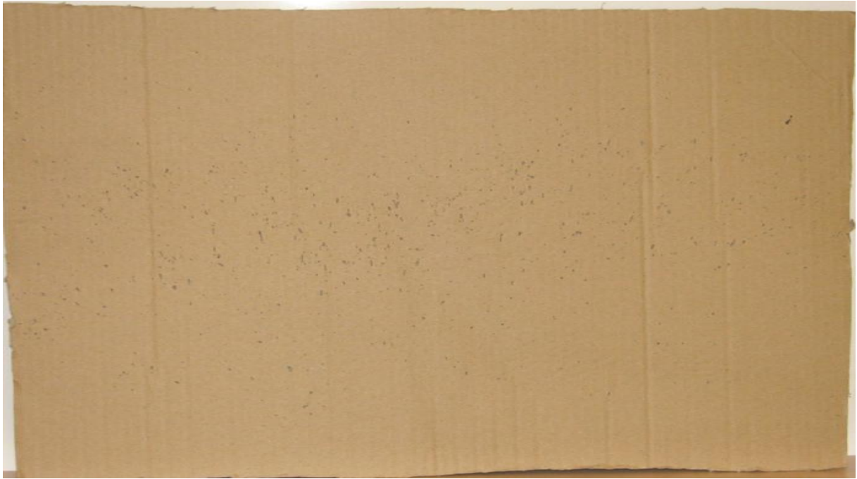
The front of the cardboard sheet. Clearly, there are no large fragments.
