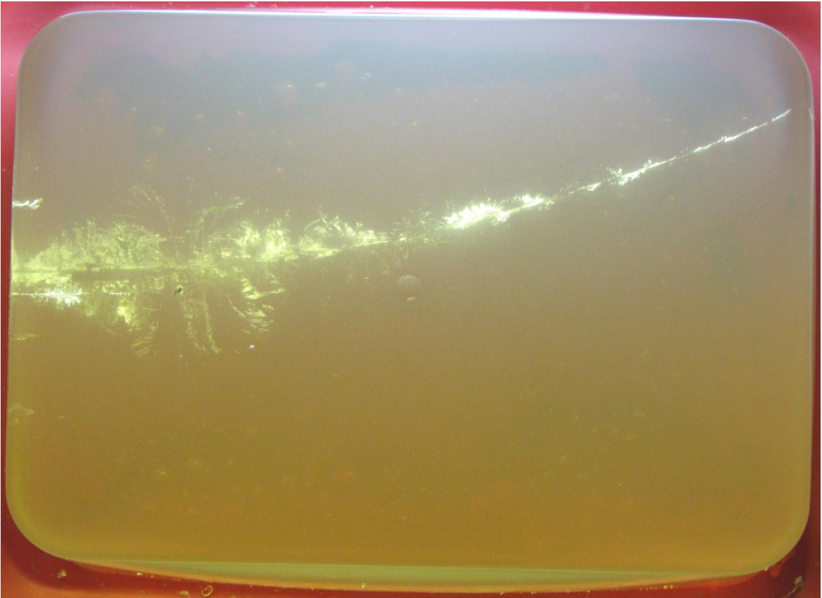
The gelatin block. The firing direction is from left to right.
