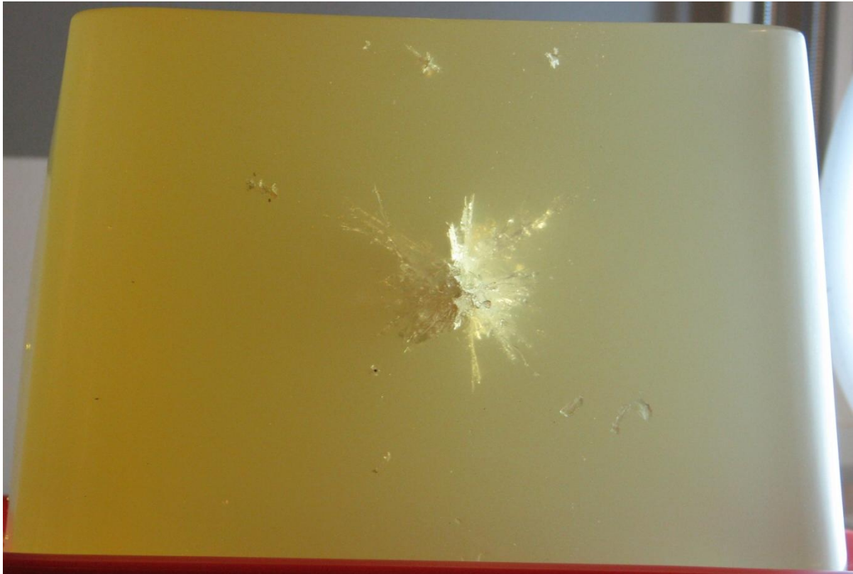
The face of the gelatin block. The distance between the point of aim and the point of impact is very small.
