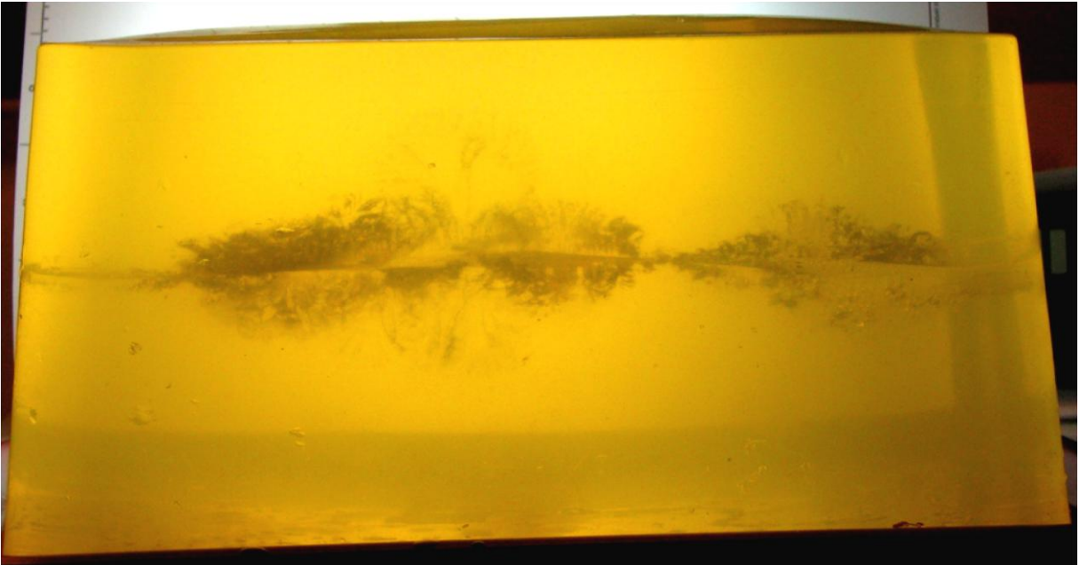
The gelatin block for shot 2, V_0 : 840m/s. Firing direction is from left to right.
