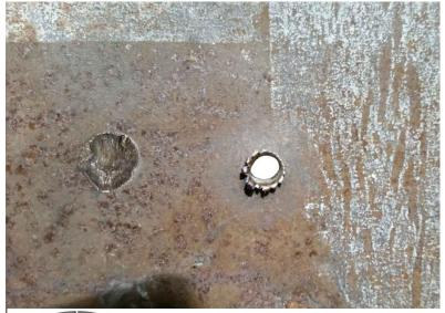
The 18mm armor plate (HB300) shown in the picture to the left shows another performance test of the 7.62x51 CBJ. It was shot at 10m range with the 7.62x51 CBJ (right hit) and left hit is from an M80 ball at the same range.
