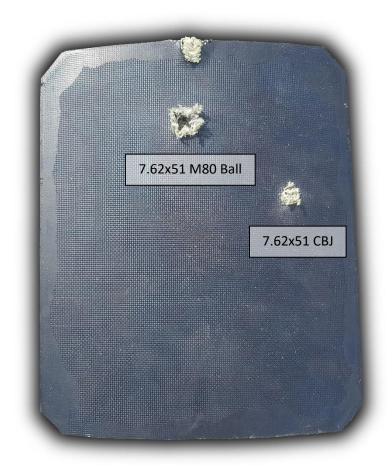
The 7.62x51 CBJ is still under development and the performance is continuously being evaluated. Apart from the ballistic performance a lot of focus is on the penetration performance against different kinds of barriers between the shooter and the intended target.
