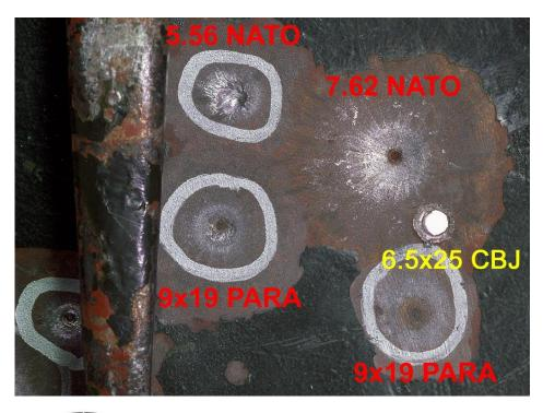
Several tests have also been done against thinner armor plates, like the one below which has been used in previous testing with the 6.5x25 CBJ Ball.
