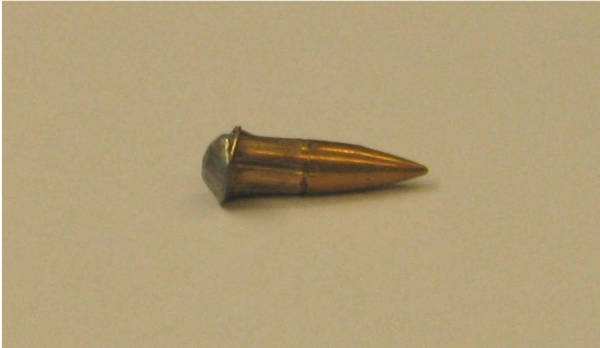
Figure 8: The projectile of shot 2. The bullet is slightly deformed, but has not fragmented.
