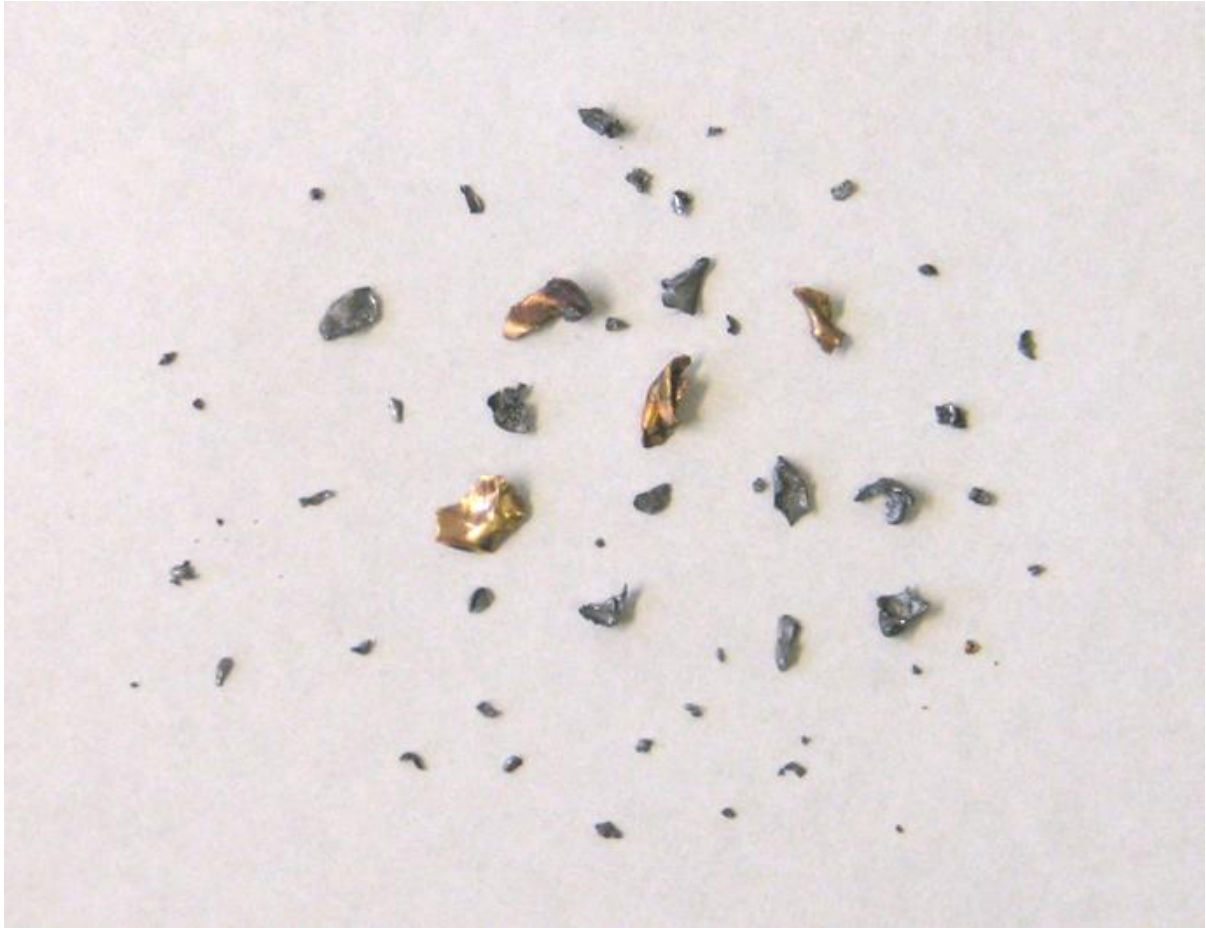
Figure 5: Fragments recovered from the gelatin block after shot 1. Weight: 20,5gr.
