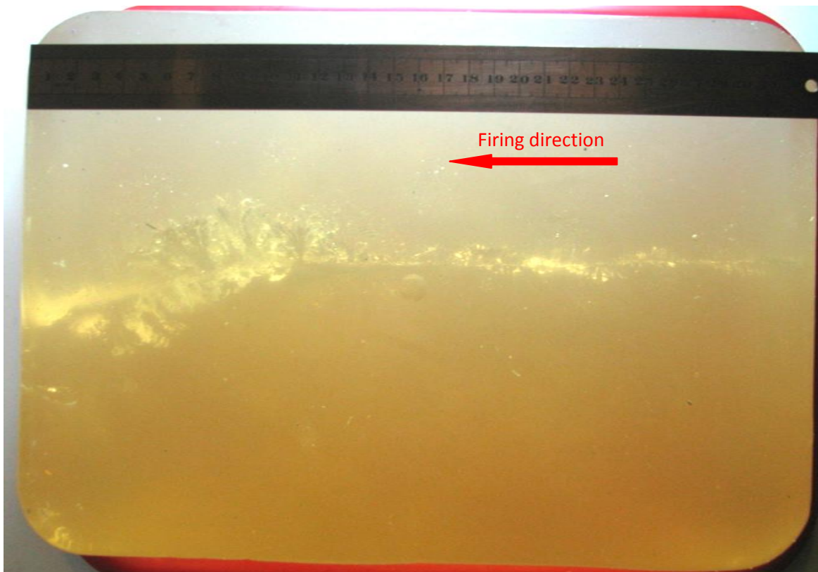
Figure 6: Gelatin block after shot 2. Note the minimal tissue disruption of the first two thirds of the bullet path.
